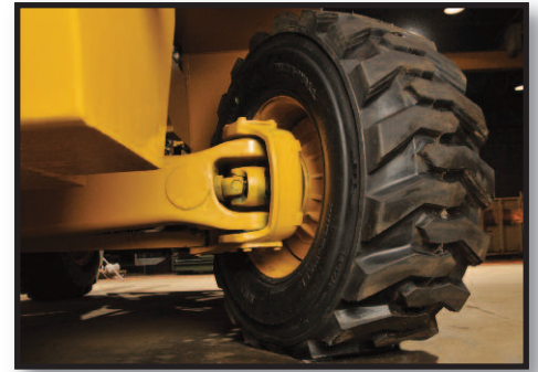
STEERING CONTROL: Designed for durability and performance with an oversized axle featuring high steer angle and heavy duty spindles.
