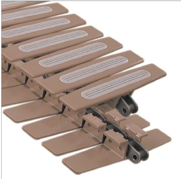
Photo shows 1873 TAB SuperGrip TableTop Chain with High Friction Inserts and top plates molded in Low Friction (LF) material on Carbon Steel (S) base chain.
